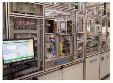
Vision Stone developed and installed a custom-made vision inspection system for TRW with multiple smart cameras from Microscan.
